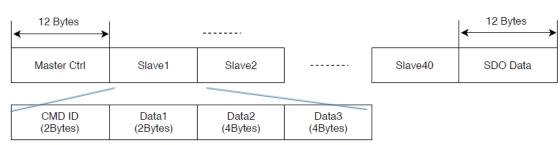
The data size of SPI transmit/receive for each slave will be 16 bytes if the CONFIG2 pin has pull-high, and the maximum 30 slaves will be control. For the detail definition of the data, please refer to the "ECM-SK Quick Start Guide"
