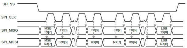
Complete SPI transmit/receive data should be 504 or 512 bytes depend on CONFIG2 pin. The data size of SPI transmit/receive for each slave will be 12 bytes if the CONFIG2 pin has pull-low, and the maximum 40 slaves will be control.
